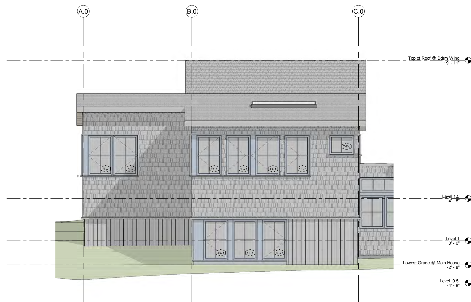
2 Exterior Elevation_South @ Bdrm Wing 3/16" = 1'-0"
