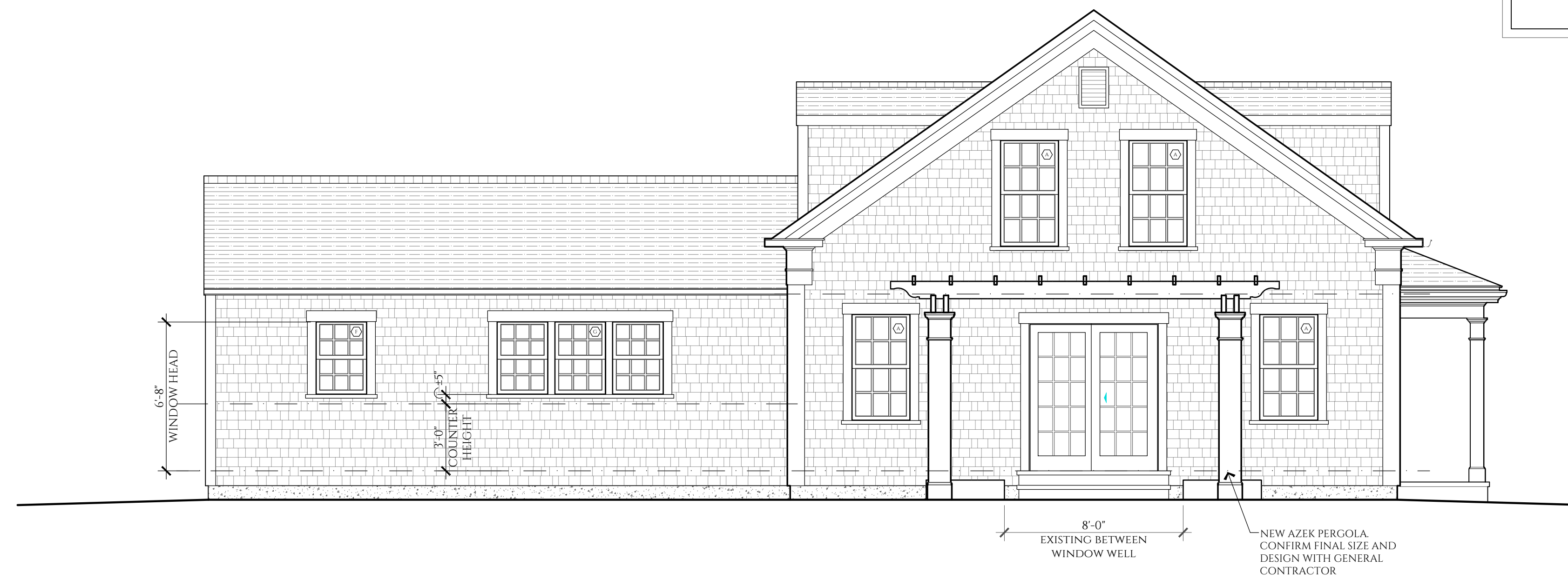
2 GUEST HOUSE - LEFT SIDE EXTERIOR ELEVATION SCALE: 1/4"=1'-0"
